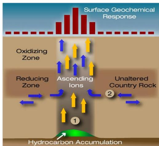
**This diagram shows an ionic plume, generated over oil & gas pools, migrating vertically to the surface**
